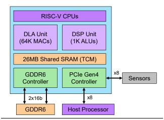
**Figure 1. Vsora's Tyr 1 chip.** The DLA units can generate 256 TOPS for AI models while the DSP units generate 4 TOPS for signal processing.
